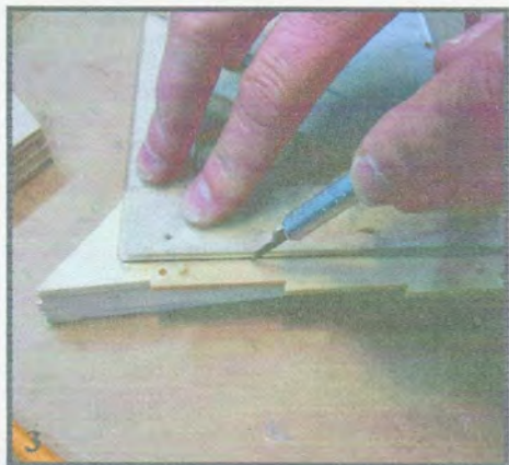
Sometimes it is easier to scribe a line on the back side of section till you cut all the way through or scribe it deep enough that you can snap off the piece.
